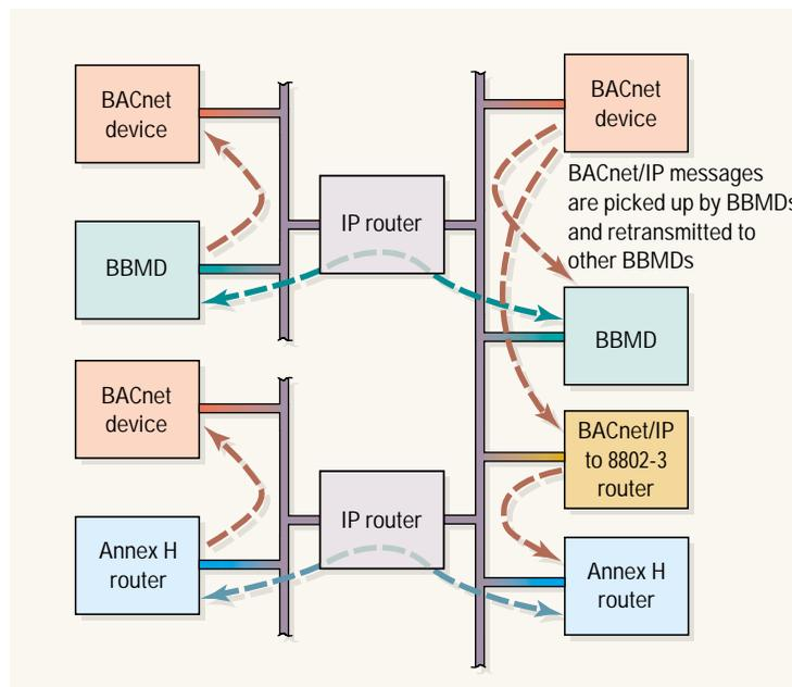
**Figure 7.** Integrating networks having mixed types of BACnet devices and mixed network technologies can be very complex, requiring different types of routers.
