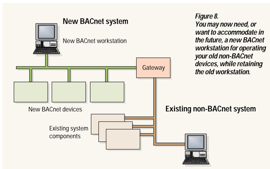
**Figure 8.** You may now need, or want to accommodate in the future, a new BACnet workstation for operating your old non-BACnet devices, while retaining the old workstation.
