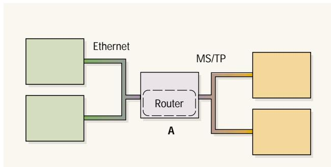
**Figure 3.** Device "A" might be a BACnet controller that also has router functionality
