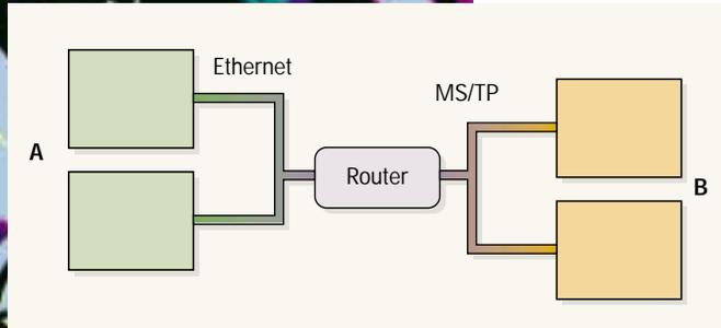
**Figure 1.** Router repeats messages from LAN "A" to LAN "B" and vice-versa, even though the two LANs are different networking technologies.
